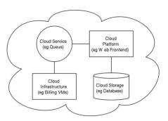
Involves multiple components communicating with each other over application programming interfaces, usually web services and 3-tier architecture.
