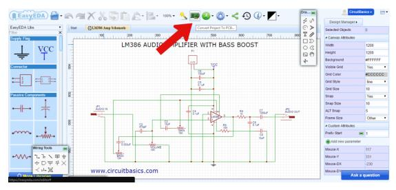
The footprints associated with each schematic symbol will be automatically transferred to the PCB editor:
