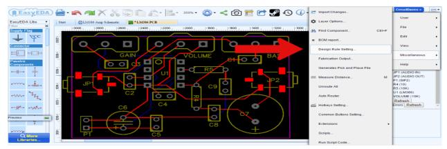
This will bring up a window where you can set design rules for trace width, distance between traces, and other useful parameters:
