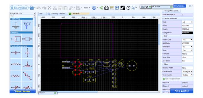
Notice the thin blue lines connecting the components. These are called *ratsnest* lines. Ratsnest lines are virtual wires that represent the connections between components. They show you where you need to route the traces according to the wiring connections you created in your schematic:
