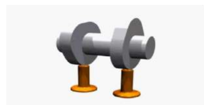
Figure 1.1 Computer animation of a camshaft operating valves
