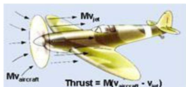
Fig:1.2 air flow through propeller
