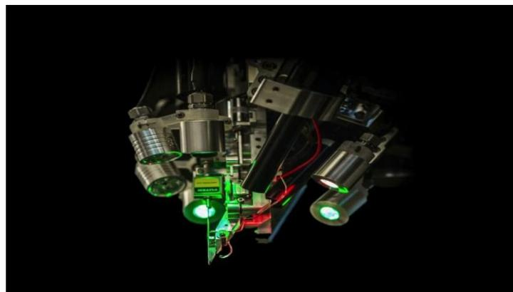
Neuralink has also created a neurosurgery robot capable of implanting the threads.
