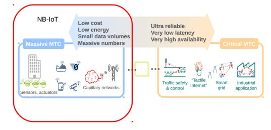
New physical layer signals and channels are designed to meet the demanding requirement of extended coverage – rural and deep indoors – and ultra-low device complexity. Initial cost of the NB-IoT modules is expected to be comparable to GSM/GPRS. The underlying technology is however much simpler than today's GSM/GPRS and its cost is expected to decrease rapidly as demand increases.
